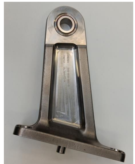
NEW BEARING INSTALLED
